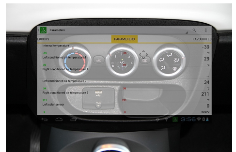
The Moverio glasses provide a mechanic with information projected onto their field of view.
